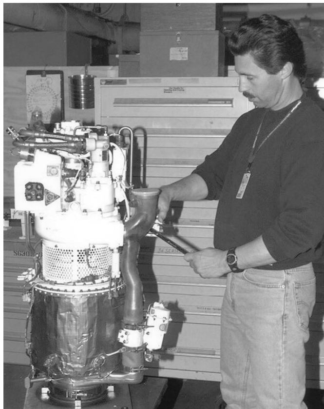
Figure 7: F/A-18 Auxiliary Power Unit Being Repaired Under a Partnership Between the Naval Aviation Depot Cherry Point and Honeywell
