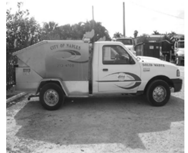
A custom designed Ranger for residential pick-up has helped reduce fuel use.
